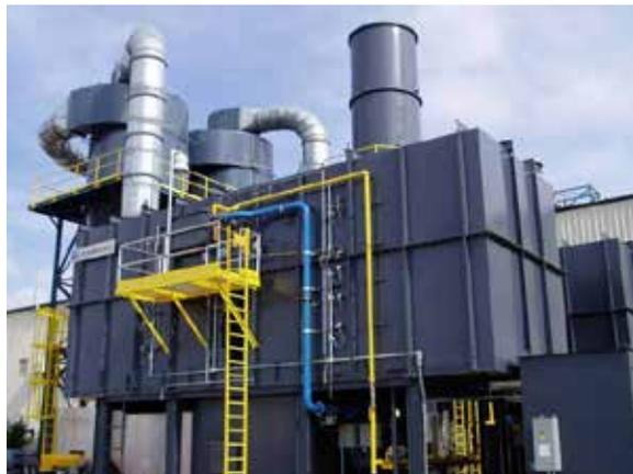
*Thermal and catalytic oxidation are the best options to destroy VOCs.*
