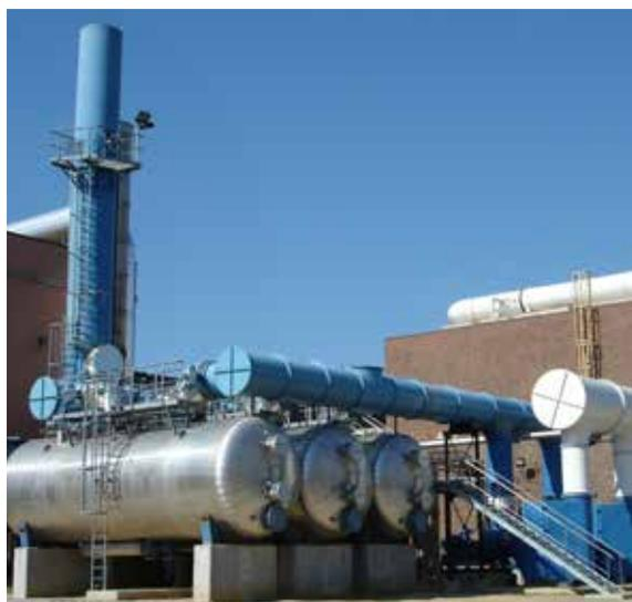
*Large carbon adsorption solvent recovery system*
