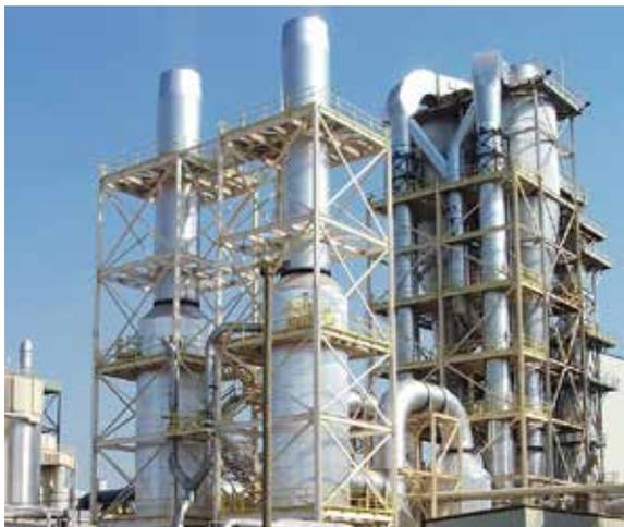
*Packed towers for gas absorption*
