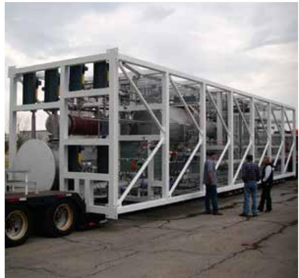
*Pre-assembled distillation system on skids*
