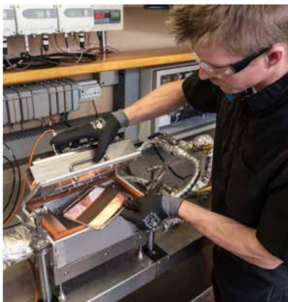
*The in-house drying lab features a bench-top system for capturing the drying behavior of coatings on web-based substrates using small-size samples approximately 5 inches by 5 inches. The drying lab allows for early scale-up steps in coating formulation development, dryer optimization, and overall process trouble shooting for coating paper, films, foils, laminates, fabrics, membranes, and other flexible web materials.*
