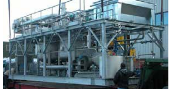
Steam regenerated adsorption to recover dichloromethane from pharmaceutical batch manufacturing plant
